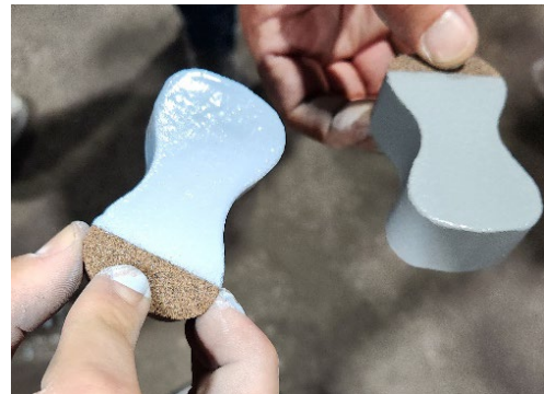
Figure 2. The dog bone test coupons after dipping.
